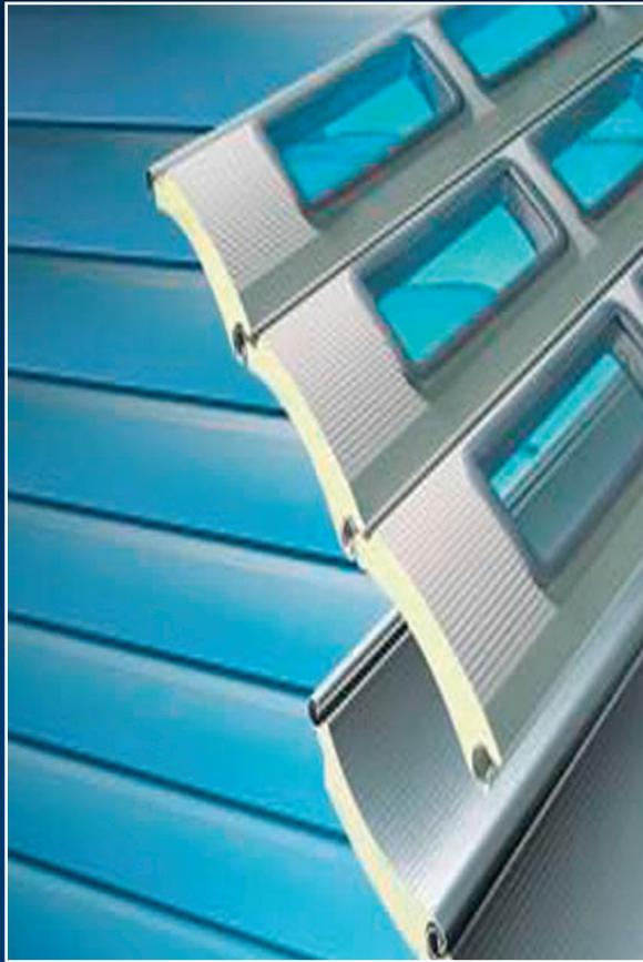
The AD95 compact insulated door offers a high quality robust and compact solution with a contemporary design suitable for all retail, commercial and industrial applications. The pu foam Filled curtain ensures minimal heat loss with maximum energy savings along with a big reduction in carbon foot print. Designed and manufactured to exact structural openings and available in galvanised as well as hard wearing and durable Laminate finishes.
